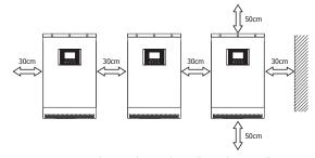
**NOTE:** For proper air circulation to dissipate heat, allow a clearance of approx. 30 cm to the side and approx. 50 cm above and below the unit. Be sure to install each unit in the same level.
