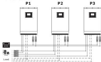
NOTE: No connect 3-phase equipment of delta connection
